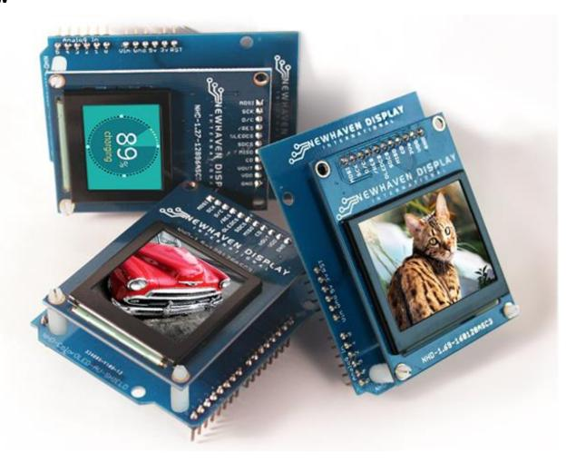
Engineered in Elgin, IL USA, the Color OLED Arduino Shields are available in three sizes: 1.27", 1.5" and 1.69" diagonal. Each Color OLED Arduino Shield comes with a serial interface color OLED display module that has a single row pinout designed for easy breadboarding, can support video, and has all the great display features of Newhaven Display's Full Color OLEDs.
