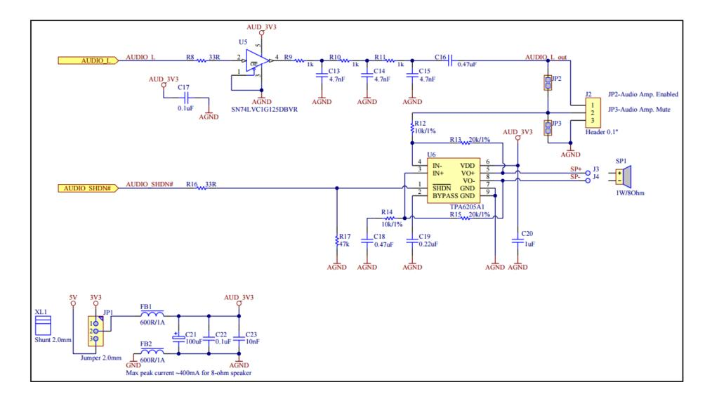
This is a reference schematic from FTDI, which can be used to successfully filter and amplify the audio signals coming from the NHD EVE TFT Module.
