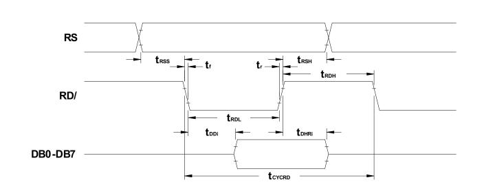
Figure 6. Intel I80-Type Parallel Interface Read Cycle Timing
