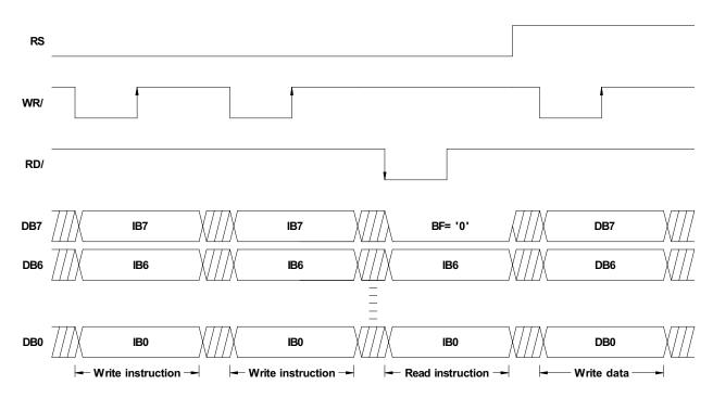
Figure 10. Typical 8-Bit Parallel Interface Sequence Using I80-Type Mode
