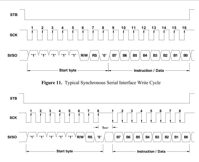
Figure 12. Typical Synchronous Serial Interface Read Cycle
